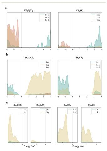
Fig. 7 Orbital-projected local electronic density of states of  $Cd_5S_4Cl_2$ ,  $Cd_4SF_6$ ,  $Sn_5S_4Cl_2$  and  $Sn_4SF_6$ . s- p- and d-orbital contributions from the metal species to the density of states near the band edges for the Cd-containing (a) and Sn-containing (b) compounds. The s- and p-orbital contributions from S and the halide species to the upper valence band for the Sn-containing compounds are also shown (c).
