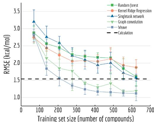
Fig. 13 Out-of-sample performances with different training set sizes on FreeSolv. Each datapoint is the average of 5 independent runs, with standard deviations shown as error bars.
