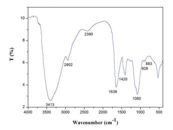
Fig. 6 FT-IR spectroscopy of NTWP-II.
