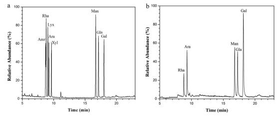
Fig. 4 The GC-MS chromatograms of derivatives of 8 standard monosaccharides (a) and component monosaccharides released from NTWP-II (b). Peaks: (1) p-Amr, (2) L-Rha, (3) p-Lyx, (4) p-Ara, (5) p-Xyl, (6) p-Man, (7) p-Gla, (8) p-Gal.
