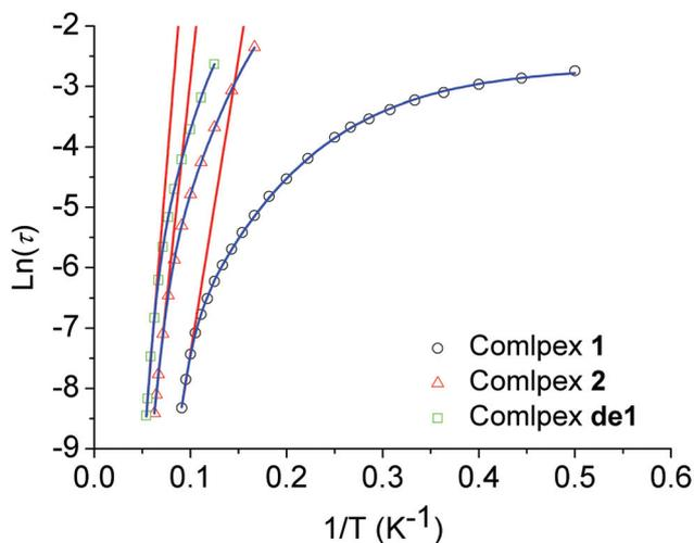
**Fig. 6** Plot of  $\ln(\tau)$  versus  $1/T$  at a zero dc field for **1**, **2** and **de1**. The red lines represent a pure Arrhenius fitting at the high-temperature linear region for **1**, **2** and **de1** at a zero dc field. The blue lines represent the fitting of the frequency-dependent data by eqn (1) for **1**, **2** and **de1** at a zero dc field.
