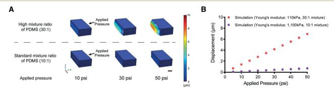
Fig. 2 Simulation results for the displacement of the actuated membrane by applying various pressures. (A) Examples of PDMS membrane deformation using different applied pressures from the results of COMSOL simulation. The color bar represents the scale of membrane displacement. Scale bar: 10 µm. (B) Red and purple represent simulation results from COMSOL Multiphysics (Young's modulus - red (30:1 PDMS mixture used in this study: 110 kPa) and purple (10:1 standard PDMS mixture: 1100 kPa)).
