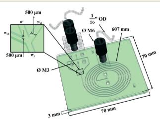
1 Microfluidic flocculation device (µFLOC). representation of the 607 mm long  $\mu$ FLOC comprising of a  $\psi$ -shaped hydrodynamic focussing inlet. The channels have an aspect ratio of 1. The width of the channel after the inlet  $(w_0)$  is 500  $\mu$ m.
