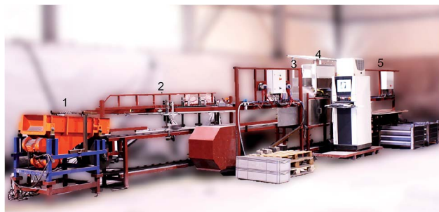
Fig. 6 Prototype sorting machine for refractories with integrated LIBS unit (material flow from left to right). (1) feeding, (2) singularisation, (3) 3D-camera, (4) LIBS unit, (5) sorting. Photo: Fraunhofer ILT at the facilities of Orbix, Genk, Belgium.
