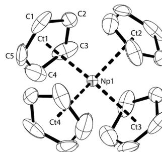
Fig. 1 Thermal ellipsoid drawing (50% probability for non-H atoms) of  $\text{NpCp}_4$  in the solid state. H atoms omitted. Selected bond lengths [Å] and angles [°] for  $\text{NpCp}_4$ : Np1–Ct 2.551(2), Np1–C 2.78(1) to 2.83(1), Ct–Np1–Ct 109.4(2).
