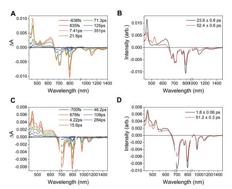
Fig. 6 Top: (A) Transient absorption spectra and (B) decay-associated spectra for PD1<sup>1-</sup>-Phbpy-Re-Py ( $\lambda_{ex} = 950$  nm). (C) Transient absorption spectra and (D) decay-associated spectra for PD1<sup>1-</sup>-Phbpy-Re-Py ( $\lambda_{ex} = 680$  nm).
