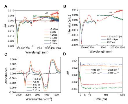
Fig. 10 (A) Transient absorption and (B) species-associated spectra for complex Phbpy-Re-PyPhNDI<sup>1-</sup> ( $\lambda_{ex} = 605$  nm) showing biphasic back electron transfer kinetics. Kinetic traces and fits are shown in Fig. S7.† (C) fsIR spectra and (D) kinetic traces with fits for complex Phbpy-Re-PyPhNDI<sup>1-</sup> ( $\lambda_{ex} = 605$  nm) showing monophasic back electron transfer kinetics. The instrument response is approximately 2 ps.
