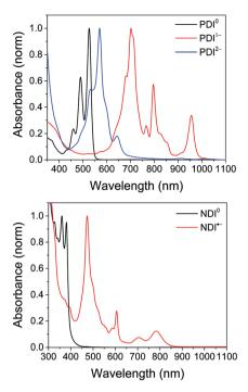
Fig. 1 Top: Spectra of PDI-Phbpy-Re-Py in the neutral (black), PDI-(red) and PDI<sup>2-</sup> (blue) states. Bottom: Spectra of Phbpy-Re-PyPhNDI in the neutral (black) and NDI- (red) states.
