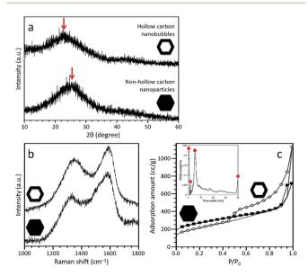
Fig. 3 (a) Wide-angle PXRD patterns, (b) Raman spectra, and (c) N<sub>2</sub> adsorption-desorption isotherms of the non-hollow carbon nanoparticles and hollow carbon nanobubbles. The pore size distribution of the hollow carbon nanobubbles is calculated by the non-local density functional theory (NLDFT) method, as shown in the inset of (c).
