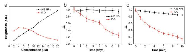
Fig. 3 Comparison between α-DTPEBBTD-C4 based AIE NPs and ICG. (a) Brightness of AIE NPs and ICG at different concentrations. (b) Fluorescence intensity changes of AIE NPs and ICG upon incubation in PBS buffer at 37 °C for 7 days. (c) Fluorescence intensity changes of AIE NPs and ICG upon irradiation with white light for 10 min.  $I_0$  and I in both (b) and (c) represent the initial and specific time point fluorescence intensities, respectively.
