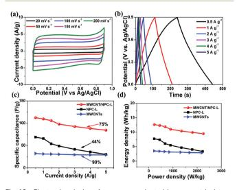
Fig. 10 Electrochemical performances evaluated by symmetrical two-electrode supercapacitors in 1 M  $\rm H_2SO_4$  solution. (a) CV curves of MWCNT/NPC-L-based SSC at different scan rates. (b) Charge–discharge curves of MWCNT/NPC-L-based SSC at various current densities. (c) Specific capacitance under different current densities from 0.5 to 5 A g $^{-1}$ . (d) Ragone plot for the SSCs based on MWCNT/NPC-L, NPC-L and MWCNTs under various current densities.
