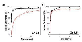
Fig. 5 Release profile of (a) calcein from Zr-L4 and (b)  $\alpha$ -CHC from Zr-L5. The crystalline MOF is presented in black closed dots and amorphous in red opened dots. Black solid and red dotted lines represent the kinetic of delivery fitting using non-linear regression on crystalline and amorphous MOFs, respectively
