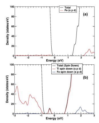
Fig. 7 (a) Spin-down DOS of  $TiO_2(R)$ -Fe. (b) Spin-down DOS of electron polaron structure of TiO2(R)-Fe. The red line represents projection of Fe states, blue line projection of Ti states. For both figures, the zero of the x-axis is fitted to the top of the VBM.
