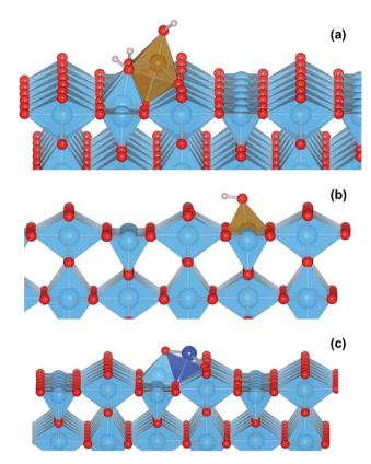
Fig. 6 (a) Final atomic structure of model TiO<sub>2</sub>(R)-Fe system, red spheres are oxygen atoms, blue spheres are titanium atoms, and brown spheres are iron atoms. (b) Final atomic structure of model  $TiO_2(R)$  –  $Fe(V_{Ti})$  system. (c) Final atomic structure of model  $TiO_2(R)$  – Cusystem, dark blue spheres are copper atoms. Prominent in all structures are the protruding twofold coordinating oxygen atoms of the ideal rutile surface
