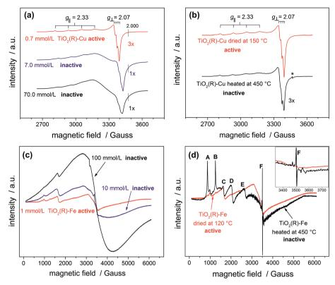
Fig. 5 EPR spectra of photocatalytically active and inactive  $TiO_2(R) - Cu$  (a) and  $TiO_2(R) - Fe$  (c) powders prepared using different concentrations of metal ion precursors; change of EPR spectra of  $TiO_2(R)$  – Cu (b) and  $TiO_2(R)$  – Fe (d) upon heat treatment at 450 °C
