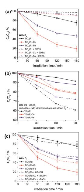
Fig. 11 Comparison of 4-CP degradation yields during photocatalytic degradation experiments using suspensions of  $TiO_2(R)$ ,  $TiO_2(R)-Cu$ and  $TiO_2(R)$  – Fe under different conditions: in the presence or absence of oxygen and in the presence of scavengers: (a) EDTA (holes), (b) tetranitromethane (electrons), (c) and tert-butanol (OH radicals). Note that the experiments in (b) have been performed in a reactor setup different from (a) and (c)
