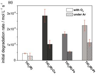
Fig. 2 Comparison of 4-CP degradation monitored by UV-Vis spectroscopy (a) (for UV-Vis absorption spectra see ESI, Fig. S5†), complete mineralization followed by changes of TOC (b), and initial degradation (c) during photocatalytic degradation experiments using suspensions of  $TiO_2(R)$ ,  $TiO_2(R)-Cu$ ,  $TiO_2(R)-Fe$  and  $TiO_2(R)-Pt$  under ambient and oxygen-free conditions
