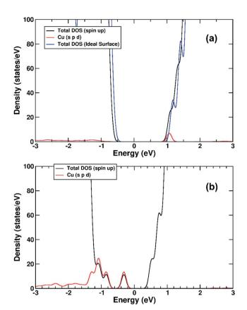
Fig. 10 (a) DOS of the  $TiO_2(R)$ -Cu system, spin-up channel only, aligned to the DOS of the ideal  $TiO_2(R)$  surface. (b) The spin up channel DOS of the final relaxed electron polaron system for the TiO<sub>2</sub>(R)-Cu system. Cu contribution shown. The zero of the x-axis is fitted to the VBM for both plots.
