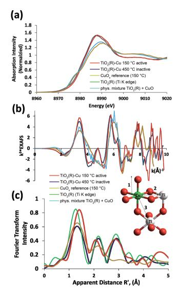
Fig. 4 XAS spectra of photocatalytically active  $TiO_2(R)$ –Cu (dried at 150 °C) and inactive  $TiO_2(R)$ –Cu (calcined at 450 °C) are compared to the reference data of  $CuO_x$  (prepared by heating), rutile  $TiO_2(R)$  (Ti K edge), and a physical mixture of  $TiO_2(R)$  and CuO. Data are presented as XANES (a), EXAFS (b) and Fourier transform of the EXAFS (c). The inset shows a structural model used for fitting.
