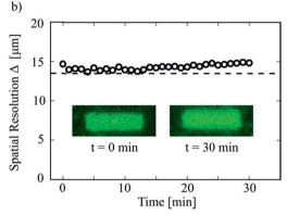
Fig. 4 Intensity profile a) of the activated pattern (inset) averaged along the direction y. The width  $\varDelta$  of the transition region (grey area) is a measure of the spatial resolution of the DROPLAY technique. The parameter  $\varDelta$  is approximately equal to the mean droplet diameter (dashed line in panel b) and slightly increases over the time due to the slow leakage of caged fluorescein across adjacent droplets. Scale bar is 50  $\mu m$ .
