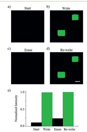
Fig. 5 Starting with a blank display (a), multiple patterns of activated droplets could be written (b), erased (c) and re-written (d) by alternating the use of the activating laser for pattern formation and excitation laser for pattern removal via photobleaching. The histogram of normalised intensities (e) - averaged over the activated regions shows that after photobleaching the pixel intensity is reduced almost to its initial value.
