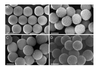
Fig. 2 Scanning electron micrographs of the SNPs; (A) native aminomodified SNPs, (B) [Cp\*Ir(biot-p-L)Cl]-S112A@prot-SNP, (C) [Cp\*Ir(biot-p- $L)Cl]\cdot S112K@prot-SNP \ and \ (D) \ [Cp*Ir(biot-p-L)Cl]\cdot S112A-K121A@prot-SNP. \\$
