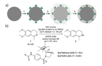
Fig. 1 (a) Immobilization and protection of ATHase in a protective organosilica layer yielding active and protected nanoparticles. The ATHase is covalently anchored (1) on the surface of SNPs (dark grey), followed by self-assembly and polycondensation of silanes (2), which eventually build a protective layer (3). (b) ATHase of cyclic imine and structure of the iridium cofactors.
