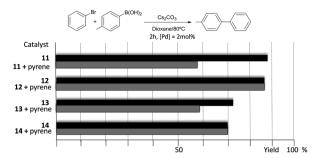
Fig. 3 Comparison of the catalytic activities of complexes 11-14 in the C-C Suzuki-Miyaura coupling of bromobenzene and p-tolylboronic acid. Grey bars indicate the activities in the presence of 10 mol% of pyrene.
