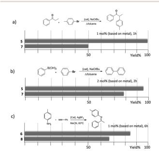
Fig. 2 Comparison of the catalytic activities of the trimetallic complexes 5 and 6 with their monometallic analogues 7 and 8. The palladium complexes were tested in the  $\alpha$ -arylation of alkylaryl ketones (a) and in the C-C Suzuki-Miyaura coupling of aryl halides with aryl boronic acids (b). The gold complexes were tested in the hydroamination of terminal alkynes with aryl amines (c)
