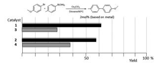
Fig. 1 Comparison of the catalytic activity of the dimetallic complexes 1 and 2, with the related monometallic analogues 3 and 4, in the C-C coupling of p-methoxyphenylbromide and p-tolylboronic acid
