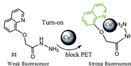
Fig. 28 Chemical structure of ligand 32 , proposed ligand–metal complexation mechanism and colorimetric change in the solution upon copper complexation.
