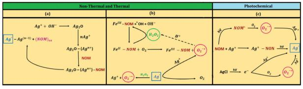
Proposed reaction mechanisms for the generation of Ag nanoparticles in the natural environment (NOM – natural organic matter)
