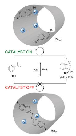
Scheme 48 Control over the activity of heterogeneous catalyst **160** through the reversible redox cleavage or formation of disulfide bonds.<sup>84</sup>
