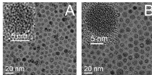
Fig. 22 TEM images of (A) core-only NaYF<sub>4</sub>:Yb,Er UCNPs and (B) core-shell UCNPs NaYF<sub>4</sub>:Yb,Er@NaYF<sub>4</sub>. The increase in diameter is attributed to the growth of an undoped host material shell on the surface of the core-only UCNPs. Reprinted with permission from ref. 70. Copyright © 2007, American Chemical Society.
