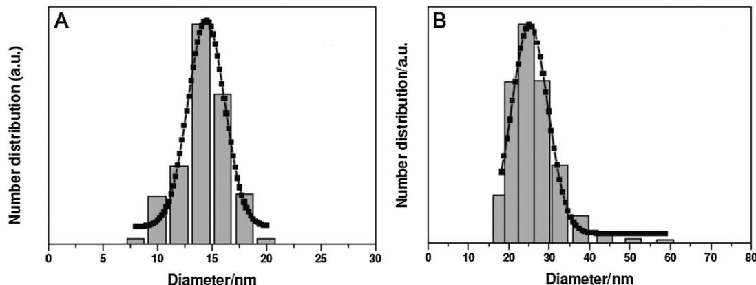
Fig. 27 DLS of UCNPs coated with oleylamine (A) and 6-aminohexanoic acid (B). The increase of the hydrodynamic diameter can be attributed to ligand change on the UCNP surface from hydrophobic (low hydrodynamic diameter) to hydrophilic (high hydrodynamic diameter). Also the size distribution remains nearly unaffected indicating a surface modification without aggregation. Reprinted with permission from ref. 122. Copyright © 2011, American Chemical Society.
