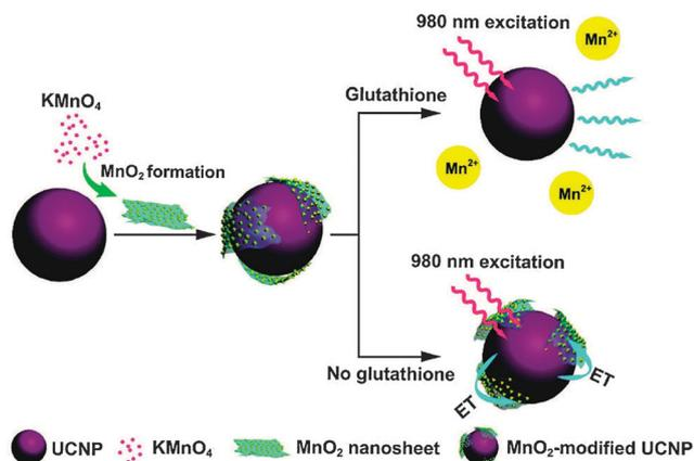
Fig. 19 Design and function of a glutathione (GSH) sensitive probe based on UCNPs. The emission of the UCNPs is quenched by the manganese oxide (MnO<sub>2</sub>) nanosheets formed on the nanoparticle surface. The analyte GSH reduces MnO<sub>2</sub>, removes the nanosheets, and restores the emission of the UCNPs. Reprinted with permission from ref. 37. Copyright © 2011, American Chemical Society.
