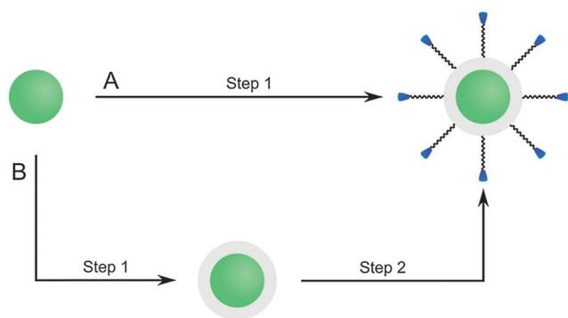
Fig. 12 Silanization by (A) growing a silica shell in presence of a functionalized silane (one-step silanization) or (B) growing a silica shell and subsequent silanization with a functionalized silane (two-step silanization).
