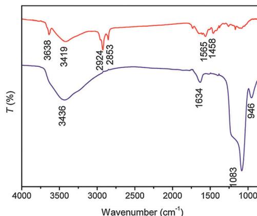
Fig. 25 FTIR spectra of unmodified  $\text{NaYbF}_4:\text{Er}$  UCNPs (upper red curve) and silica-coated  $\text{NaYbF}_4:\text{Er}$  UCNPs (lower blue curve). The strong new band at  $1083\text{ cm}^{-1}$  is assigned to stretching vibration of Si-O. Reprinted with permission from ref. 163. Copyright © 2009, American Chemical Society.
