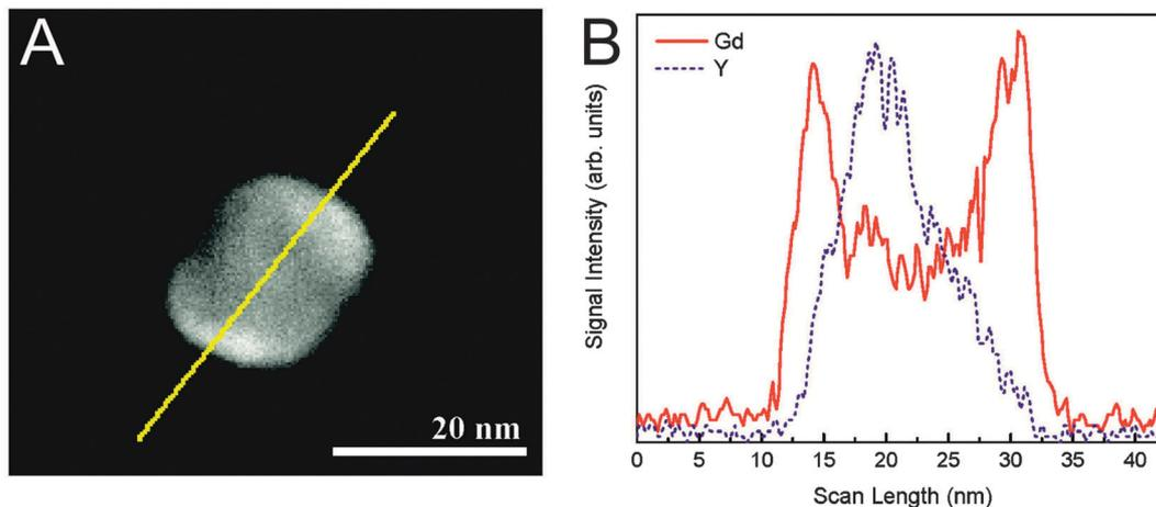
Fig. 23 (A) TEM image and (B) EDS scan of a  $\text{NaYF}_4@ \text{NaGdF}_4$  nanoparticle. The yellow line represents the scan line. The EDS scan clearly shows the different material compositions of core and shell. Reprinted with permission from ref. 67. Copyright © 2011, American Chemical society.
