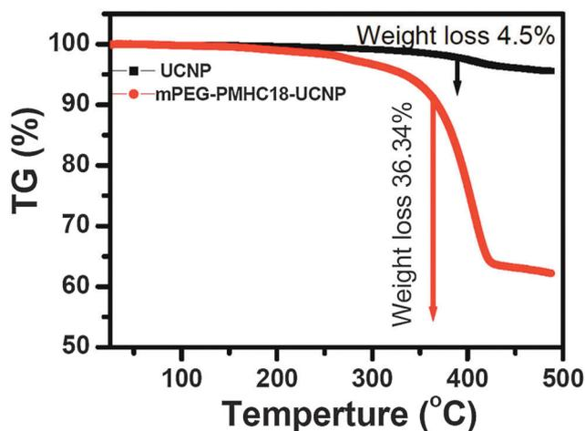
Fig. 24 Thermogravimetric analysis (TGA) curves of UCNPs coated with oleic acid (black curve) or PEG-PMHC<sub>18</sub> (red curve). The expected larger weight loss of PEG-coated UCNPs with 36.34% compared to unmodified UCNPs with only 4.5% is clearly observable. Reprinted with permission from ref. 138. Copyright © 2011, American Chemical Society.
