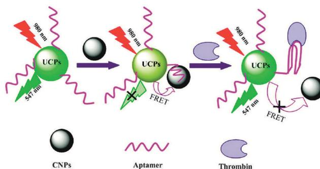
Fig. 17 Scheme of the design and function of a thrombin sensor based on UC(L)NPs. An aptamer on the UC(L)NP surface binds to a carbon nanoparticle (CNP) *via* weak  $\pi$ - $\pi$  interactions. The CNP quenches the upconversion emission by LRET. Thrombin changes the structure of the aptamer, releases the CNP from the UC(L)NP surface and thus restores the upconversion emission. Reprinted with permission from ref. 38. Copyright © 2011, American Chemical Society.
