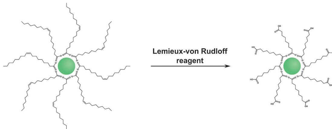
Fig. 9 Scheme of the oxidation of oleic acid with the Lemieux–von Rudloff reagent ( $\text{MnO}_4^-/\text{IO}_4^-$ ). The oxidation of the double bond leads to the formation of hydrophilic carboxylate groups on the UCNPs surface which are accessible for subsequent conjugation steps. Adapted with permission from ref. 28. Copyright © 2008, American Chemical Society.
