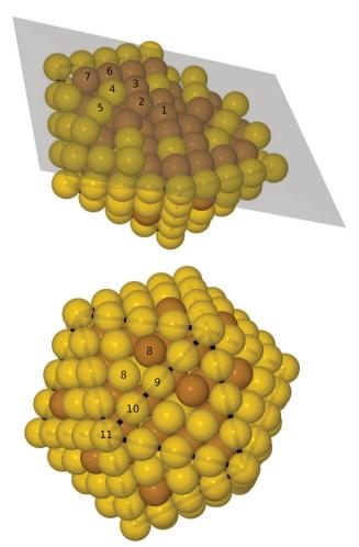
Fig. 2 Top: cut-through of the optimal particle, the numbers on the atoms indicate the subshell number. Bottom: the whole  $Au_{174}Cu_{135}$  particle. Brown: Cu, yellow: Au.
