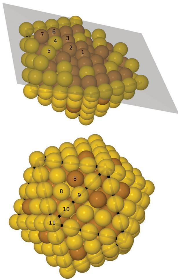
Fig. 2 Top: cut-through of the optimal particle, the numbers on the atoms indicate the subshell number. Bottom: the whole Au<sub>174</sub>Cu<sub>135</sub> particle. Brown: Cu, yellow: Au.
