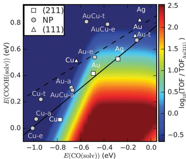
Fig. 5 Contour plot of the turn over frequency (TOF) for  $\text{CO}_2$  to CO from a kinetic model at 0.35 V overpotential.<sup>3</sup> The predicted activity of the apex, edge and terrace sites on  $\text{Au}_{174}\text{Cu}_{135}$ , Au and Cu nanoparticles from our study is shown. Activities of (111) and (211) facets are taken from ref. 64 and 2. The solid and dashed lines are trend lines for (211) and (111) surfaces, respectively, of the late transition metals.
