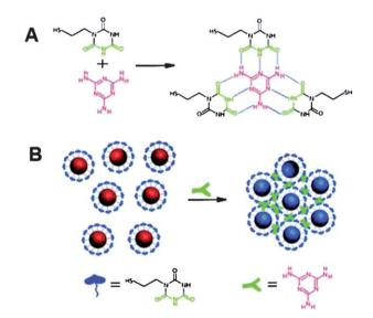
**Fig. 8** (A) Hydrogen-bonding recognition between melamine and cyanuric acid derivative. (B) Colorimetric detection of melamine using the cyanuric acid-stabilized AuNPs. Reproduced with permission from ref. 139. Copyright 2009, ACS.
