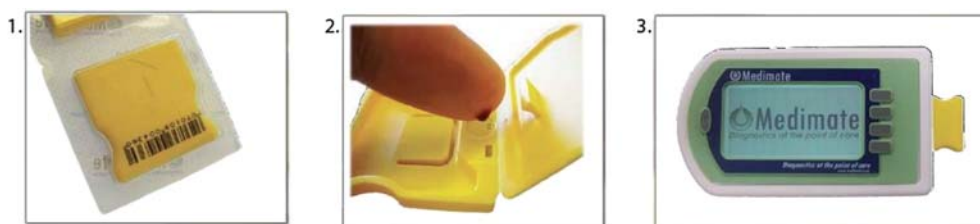
Fig. 1 (1) A cartridge containing a pre-filled microfluidic chip; (2) the cartridge is opened, the chip seal is removed and a drop of blood is deposited at the sample opening; (3) the cartridge is inserted in the Multireader and the measurement is started.
