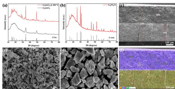
Fig. 1 XRD patterns of (a) LIC and (b) LPSC powders. SEM images of (c) ball-milled LIC and (d) LPSC powders. (e) SEM image and (f) EDS image of the cross-section of the LIC-LPSC bilayer SSE.
