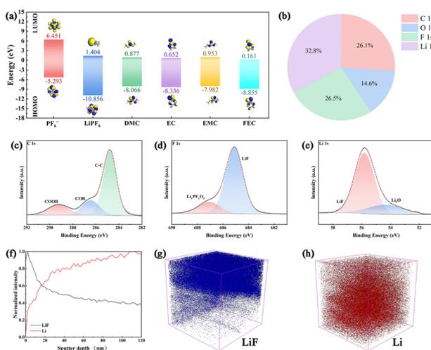
**Fig. 3** (a) HOMO–LUMO energy levels of different solvents and additives in the electrolyte. (b) Content ratio of elements distributed on the surface of FEC@Li. XPS spectrum for (c) C 1s, (d) F 1s, and (e) Li 1s of the surface of FEC@Li. (f) Normalized depth profiles of LiF and Li fragments obtained from the FEC@Li anode surface. Three-dimensional reconstruction of the ToF-SIMS sputtered volume showing the distribution of (g) LiF and (h) Li fragments within the SEI.
