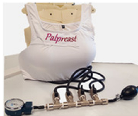
Fig. 6 Prototype design of the Palpreast device, including a smart wearable and inflator system. Reproduced from ref. 89 published under the terms and conditions of the Creative Commons Attribution (CC BY) license.
