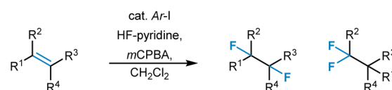
Fig. 15 Aryl iodide-catalyzed difluorination of alkenes and the two possible isomeric reaction products.
