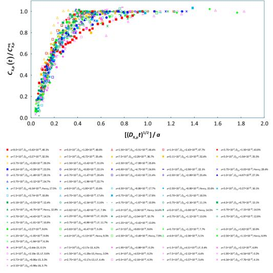
Fig. 6 Normalized kinetic sorption curves for data sets with <50% bulk depletion of the contaminant. For each data set, the legend gives the particle radius (a (m)), the intraparticulate diffusion coefficient ( $D_{X,p}$  (m<sup>2</sup> s<sup>-1</sup>)), and the % bulk depletion. Unless otherwise specified, the Langmuir isotherm is the best fit for the equilibrium data.
