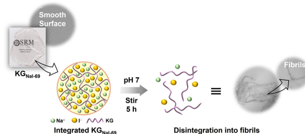
Fig. 2 Schematic representation for the biodegradability test of \text{KG}_{\text{NaI}-69} . Optical microscope image of \text{KG}_{\text{NaI}-69} film ( 10\times magnification) after immersing into aqueous medium (pH 7, stir at 200 \text{ rpm} , 5 h).
