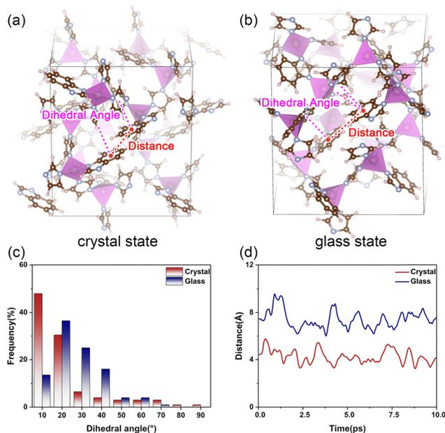
Fig. 2 (a) Representation of the ZIF-62 crystal. (b) Snapshot of the simulated ZIF-62 glass. (c) The distribution of the dihedral angles between adjacent BIM ligands in two states. (d) The evolutions of the average distances between the centers of the benzene rings in the neighboring BIM ligands in two states. The analyzed dihedral angle and distance are marked in the above figures.
