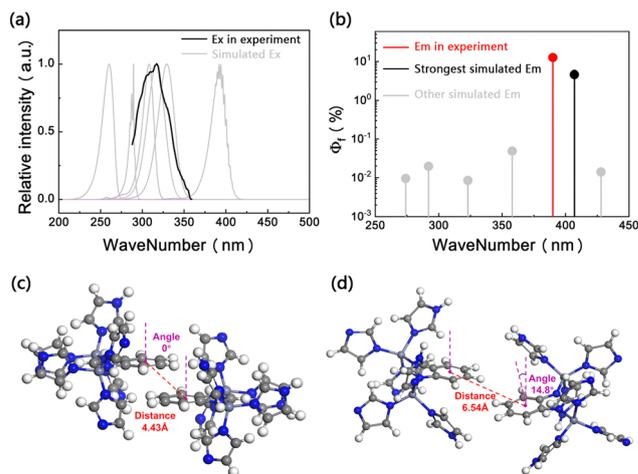
**Fig. 3** (a) The simulated absorption spectrum based on the cluster models. (b) The emission wavelengths of the examined configurations of the glassy state. (c) The arrangement of BIM ligands in the crystalline state. (d) The arrangement of the BIM ligand in the configuration with the largest  $\Phi_f$ .
