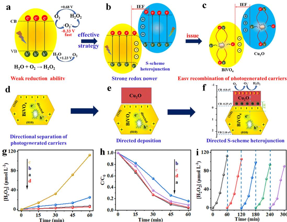
**Fig. 7** (a)–(f) Graphical illustration showing the design of the S-scheme heterojunction for highly active  $\text{H}_2\text{O}_2$  production. (g) Photocatalytic  $\text{H}_2\text{O}_2$  production and (h) time-dependent curves of photocatalytic  $\text{H}_2\text{O}_2$  decomposition of various samples. (i) Cycle test for the  $\text{MnOOH}/\text{BiVO}_4/\text{Cu}_2\text{O}$  photocatalyst. Reproduced from ref. 149 with permission from Royal Society of Chemistry, copyright 2024.
