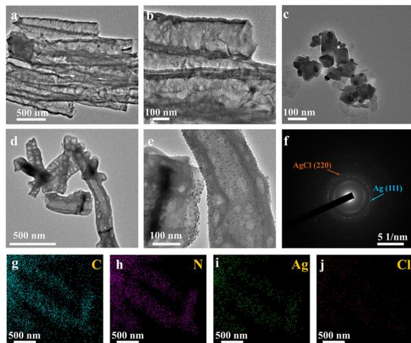
Fig. 1 TEM images of (a) and (b) GCNT, (c) AgCl, (d) and (e) AC/GCNT-2 composites; (f) SAED image and (g)–(j) mapping images of AC/GCNT-2 composites.
