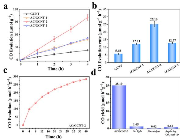
**Fig. 3** (a) The photocatalytic CO evolution performance and (b) the photocatalytic CO evolution rate of the GCNT materials and AC/GCNT-*x* composites; (c) the stability of AC/GCNT-*x* composites for photocatalytic  $\text{CO}_2$  conversion; (d) the control experiments for the photocatalytic CO evolution rate of the AC/GCNT-2 composites.
