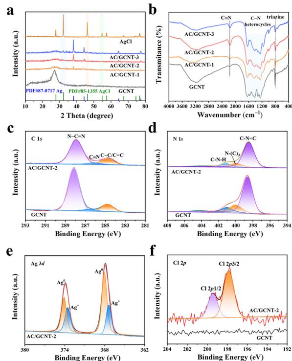
Fig. 2 (a) XRD patterns of GCNT, AgCl and AC/GCNT-*x* composites, and (b) FT-IR spectra of GCNT and AC/GCNT-*x* composites; XPS spectra of GCNT and the AC/GCNT-2 composites: (c) C 1s, (d) N 1s, (e) Ag 3d and (f) Cl 2p.
