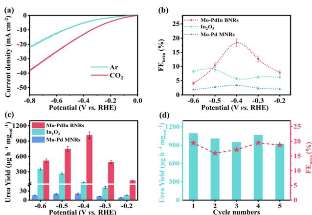
Fig. 3 (a) LSV curves of Mo–PdIn BNRs in a 0.1 M  $\text{KNO}_3$  solution with Ar or  $\text{CO}_2$  gas bubbling, respectively. (b) FE of urea and (c) urea yield of various catalysts at different applied potentials. (d) Urea yield and corresponding FEs of five independent cycles at  $-0.4$  V vs. RHE, with each cycle of 2 h.
