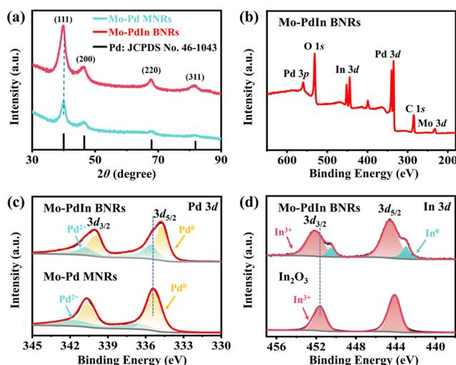
**Fig. 2** (a) XRD patterns of Mo-PdIn BNRs and Mo-Pd MNRs. (b) XPS survey spectrum of the Mo-PdIn BNRs. (c) Pd 3d XPS spectra of Mo-PdIn BNRs and Mo-Pd MNRs. (d) In 3d XPS spectra of Mo-PdIn BNRs and In<sub>2</sub>O<sub>3</sub>.
