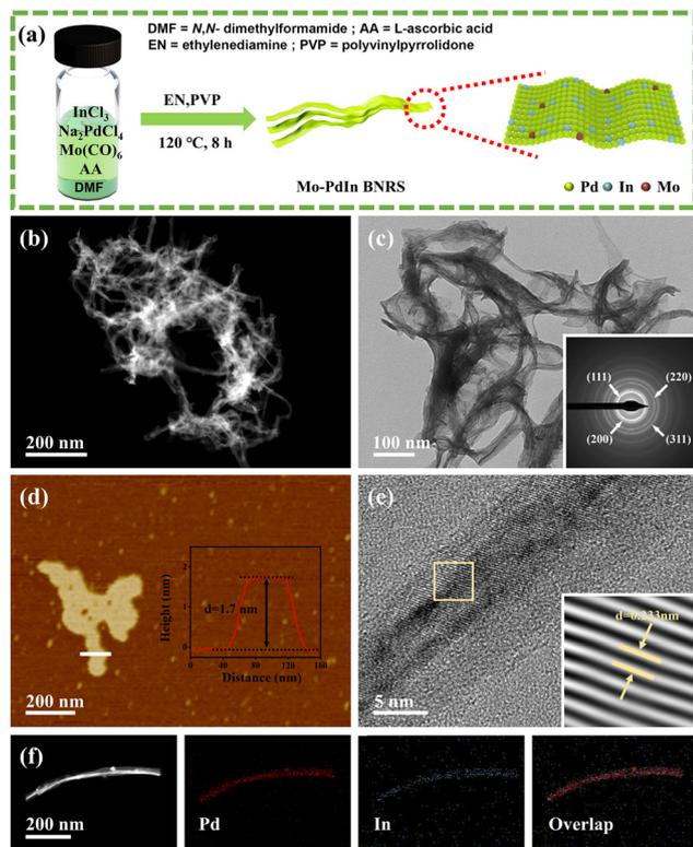
**Fig. 1** (a) Schematic diagram of the synthetic process for Mo-PdIn BNRs. (b) HAADF-STEM image, (c) TEM image and SAED pattern, (d) AFM image and relevant height profile, (e) HRTEM image, (f) HAADF-STEM image and relevant EDX mappings of Mo-PdIn BNRs. The insets in (e) show the lattice fringes of the square region.
