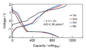
Fig. 4 Charge-discharge profiles for all-solid-state fluoride battery with metallic Mn electrode in ranges of -2 V to 2 V (starting from fluorination of metallic Mn). Cell structure is Pb/PbF2-SnF2-AB/BLF/Mn-BLF-AB. The capacity was calculated based on the weight of Mn
