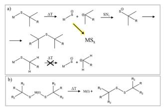
Fig. 4 (a) Thermal decomposition of thiols and formation of MS<sub>x</sub> nanomaterials. Figure adapted from ref. 79 under Creative Commons Attribution licence CC BY 4.0 (b) redox reaction of thiols and metals reported in ref. 86.
