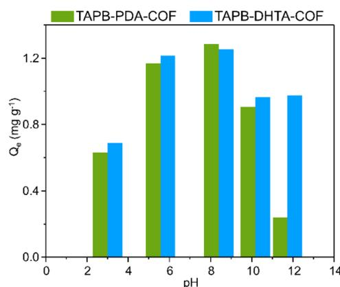
Fig. 2 Q<sub>e</sub> of TAPB-PDA-COF and TAPB-DHTA-COF towards Fe<sup>2+</sup> depending on the pH of the media.
