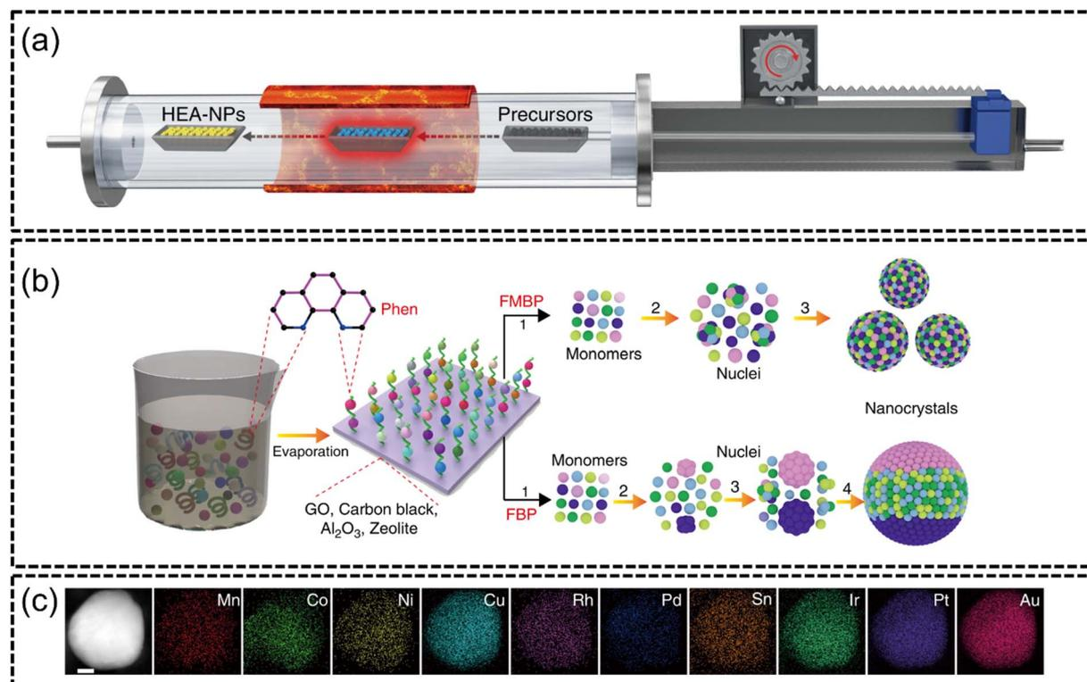
Fig. 6 FMBP synthesis from the work of Gao *et al.*, (a) illustration of the FMBP experimental setup to synthesize HEA NPs from precursors, (b) schematics for the synthesis of HEA NPs which are homogeneous when synthesized *via* FMBP, and phase-separated when synthesized *via* fixed bed pyrolysis (FBP), and (c) STEM-EDX elemental mapping of MnCoNiCuRhPdSnIrPtAu constituents. The scale bar is 10 nm. Reproduced with permission.<sup>105</sup> Copyright Springer Nature 2020.
