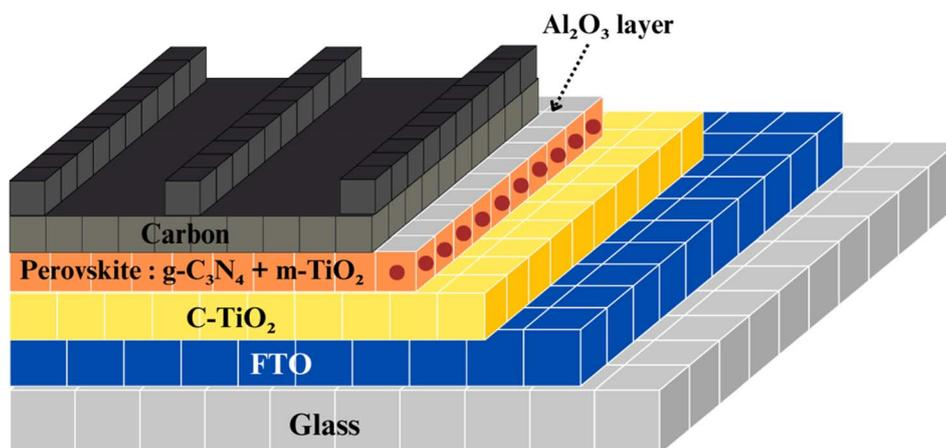
Fig. 22 Al<sub>2</sub>O<sub>3</sub> layer insulated g-C<sub>3</sub>N<sub>4</sub> added carbon-based perovskite solar cells.
