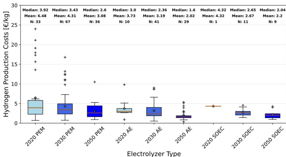
Fig. 7 Boxplots of hydrogen production costs *via* electrolysis for different production technologies. "\*" represents the arithmetic mean. "+" represents outliers. PEM = Polymer Electrolyte Membrane, AE = Alkaline Electrolysis, SOEC = Solid Oxide Electrolysis Cells.
