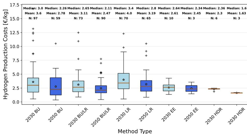
Fig. 10 Boxplots of hydrogen production costs for different forecasting methods. "\*" represents the arithmetic mean. "+" represents outliers. BU: bottom-up analysis, BU/LR: combination of bottom-up analysis and learning curve approach, LR: learning curve approach, EE: expert elicitation, HDR: historic data regression.
