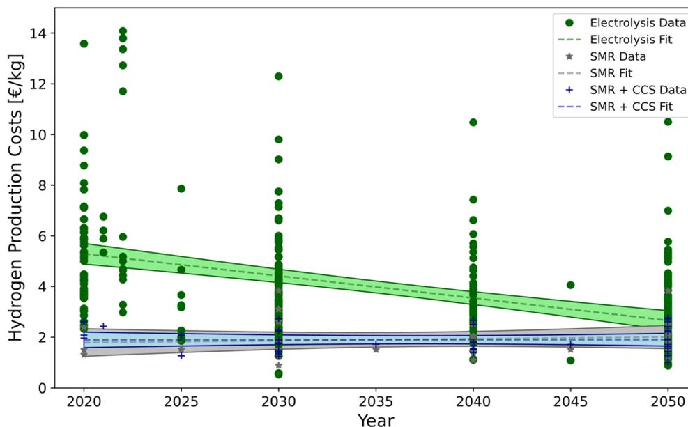
Fig. 12 Scatter plot showing the predicted production costs for different hydrogen production technologies and a corresponding linear fits. The colored frames indicate the 95% confidence interval.
