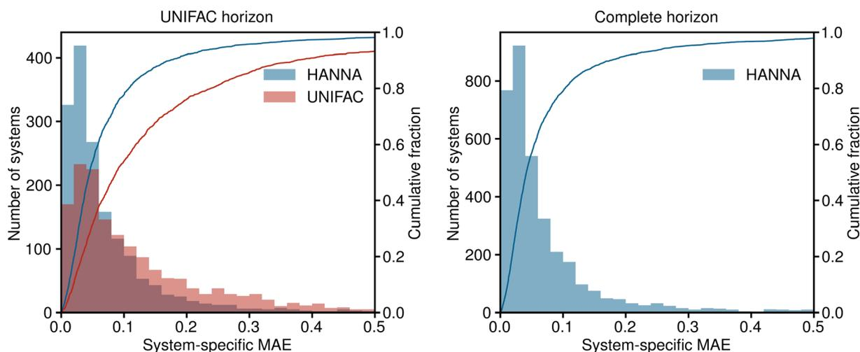
Fig. 3 Histograms and cumulative fractions showing the system-specific MAE for predicting logarithmic activity coefficients  $\ln \gamma_i$ . Left: comparison of HANNA with UNIFAC on those test data that can be predicted with UNIFAC (UNIFAC horizon). The shown range covers 98.1% of the predictions of HANNA and 93.2% of the predictions of UNIFAC. Right: results of HANNA on the complete test set. The shown range covers 97.9% of the predictions.
