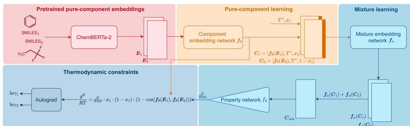
Fig. 1 Scheme of HANNA, the first hard-constraint NN for predicting activity coefficients in binary mixtures. Technical details on the architecture are given in Section *Data splitting, training, and evaluation of the model*.
