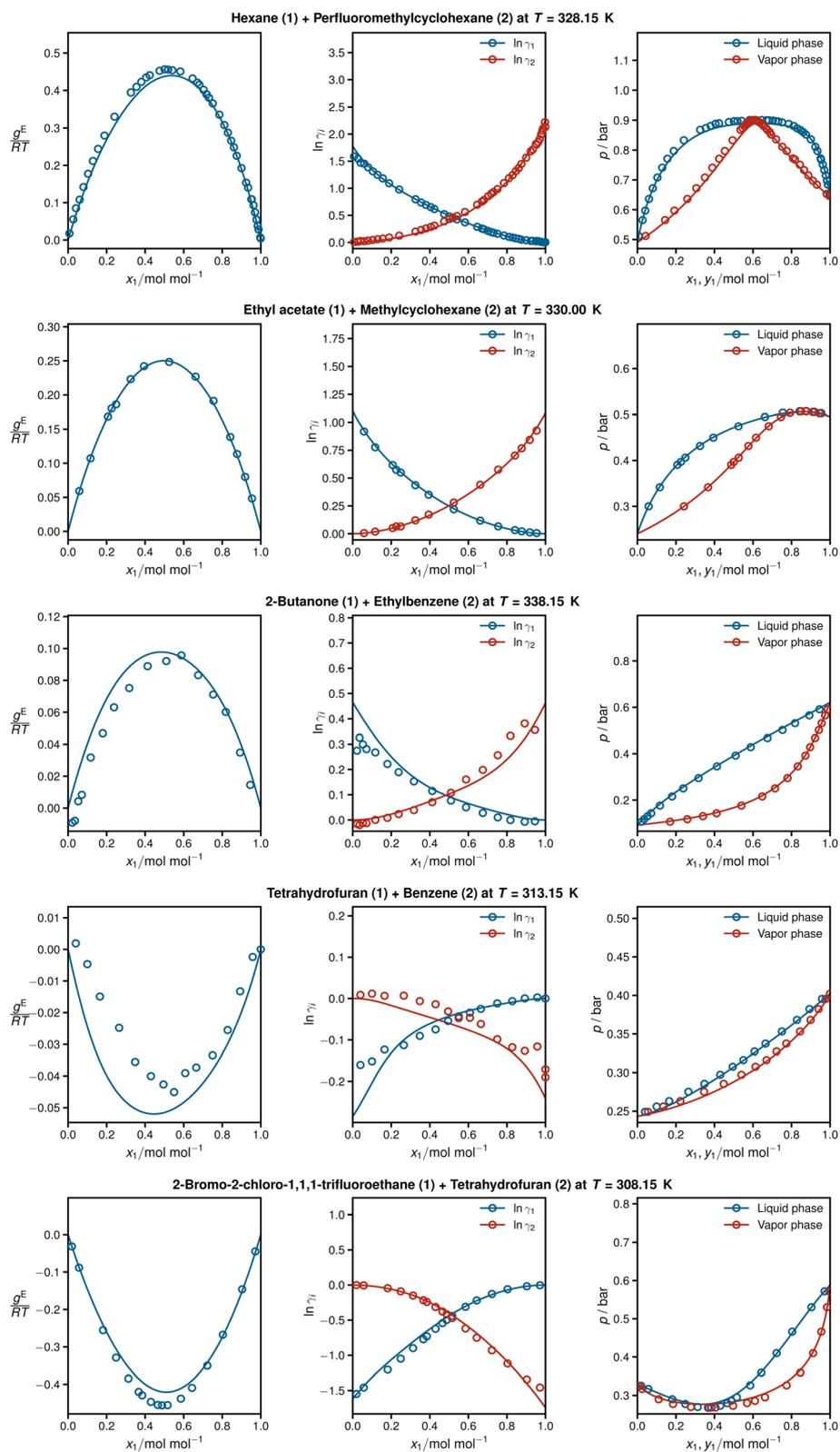
Fig. 4 From left to right: Gibbs excess energies  $\frac{g^E}{RT}$ , resulting logarithmic activity coefficients  $\ln \gamma_i$ , and isothermal vapor–liquid phase diagrams for five systems from the test set plotted as a function of  $x_1$  as predicted with HANNA (lines) and comparison to experimental test data from the DDB<sup>70</sup> (symbols). No data for any of the depicted systems were used for training or hyperparameter optimization.
