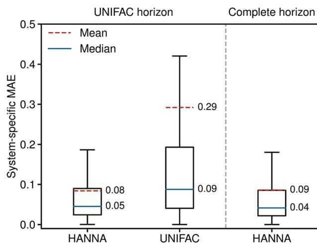
Fig. 2 System-specific MAE of the predicted logarithmic activity coefficients  $\ln \gamma_i$  from HANNA and UNIFAC. Left: results for those data from the test set that can also be predicted with UNIFAC (UNIFAC horizon). Right: results for the complete test set (complete horizon).
