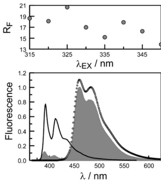
Fig. 9 The lower panel compares the fluorescence spectrum recorded for PY-P<sub>8</sub>-PER in chloroform (shaded profile) following excitation at 350 nm with spectra projected for  $P_{\text{EET}}$  values of 0% (black curve) and 100% (open circles). The upper panel illustrates how the ratio of integrated emission profiles depends on excitation wavelength.
