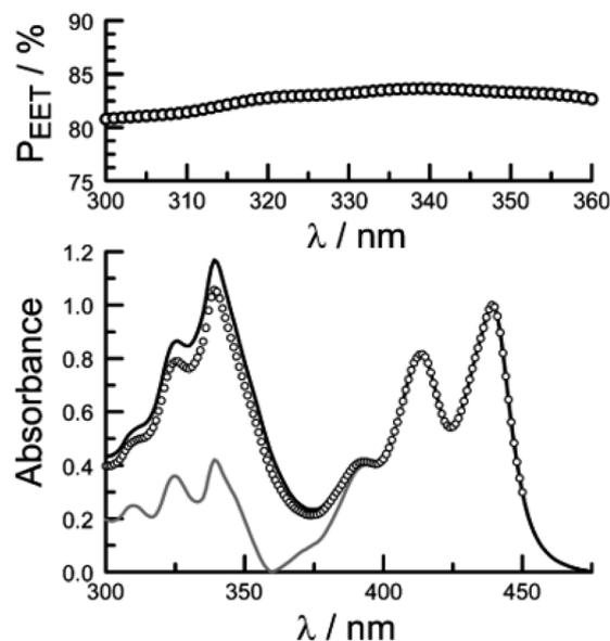
Fig. 8 The lower panel shows a comparison of normalised absorption (black curve) and excitation (open circles) spectra recorded for **PY-P<sub>8</sub>-PER** in dilute chloroform solution. The fluorescence wavelength was 525 nm. The grey curve represents the absorption spectrum derived for the perylene component of the dyad. The upper panel shows the wavelength dependence for  $P_{EET}$  as measured by this procedure, the median value being 83%.
