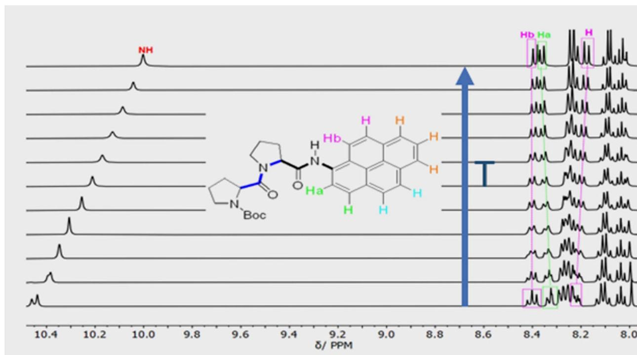
Fig. 3 Variable temperature  $^1\text{H}$  NMR spectra of **PY-P<sub>2</sub>** in  $\text{D}_6$ -DMSO showing the aromatic region and the most downfield proton resonances. The blue arrow indicates the direction of increasing temperature. The first spectrum was recorded at 298 K, the second at 313 K and subsequent spectra were recorded at intervals of 10 K until 403 K.
