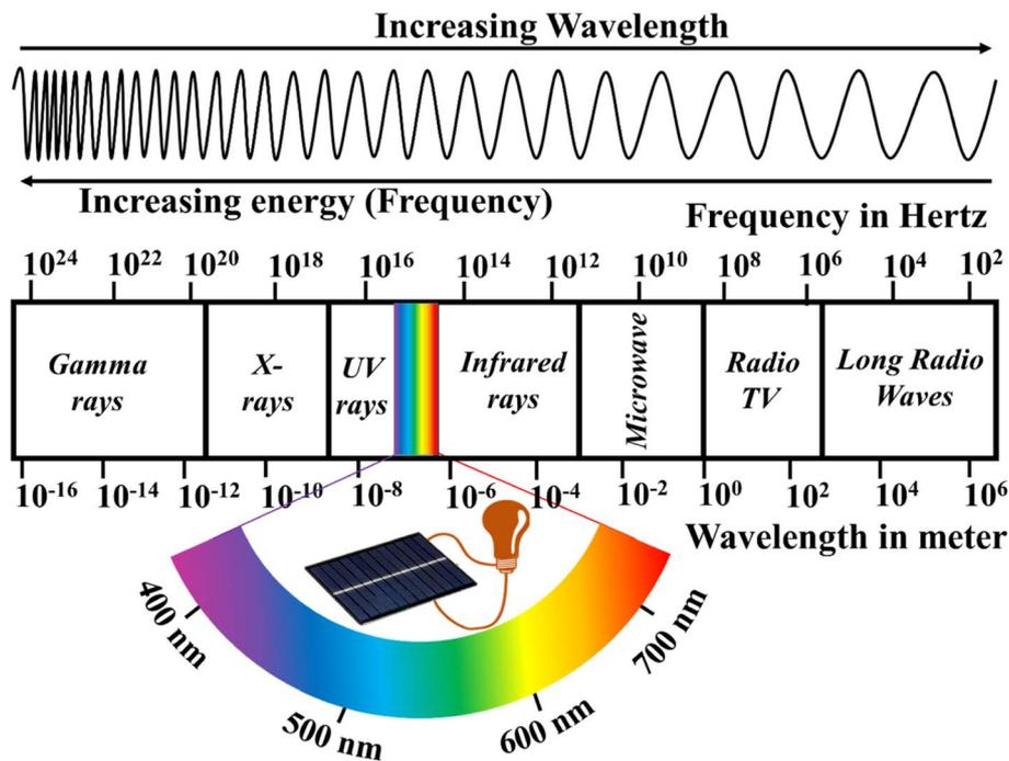
Fig. 4 Solar energy spectrum.
