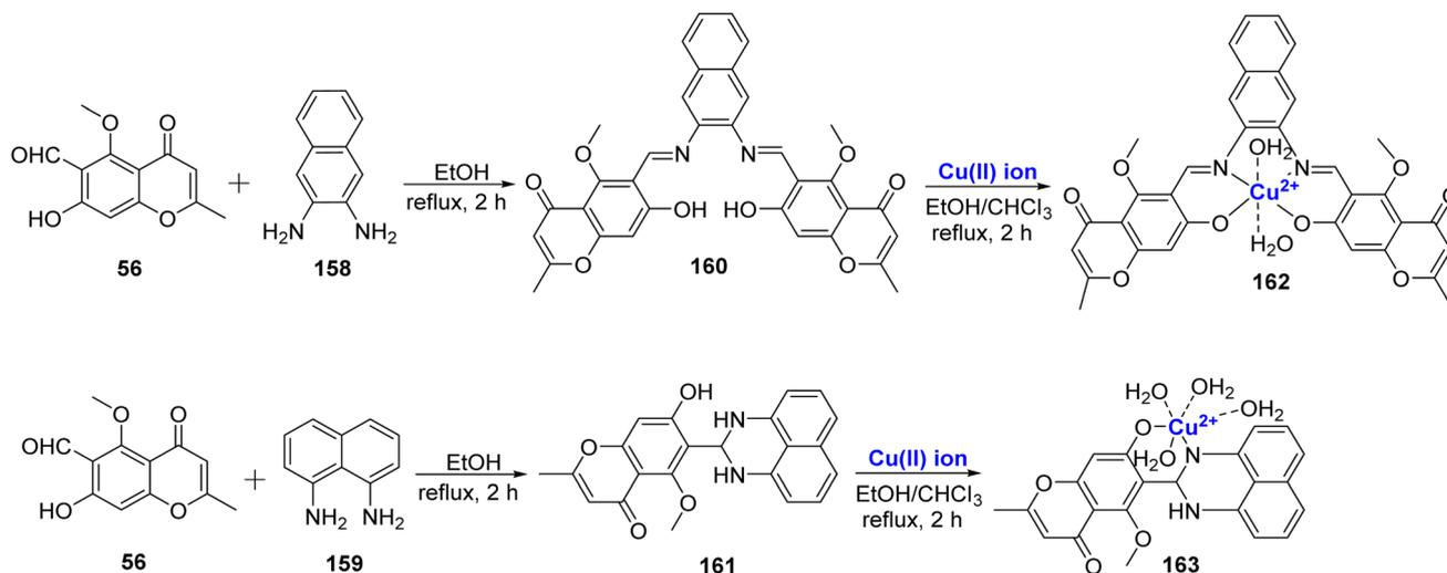
Scheme 49 Synthesis of ligands **160–161** and Cu(II) ion complexes **162–163**.
