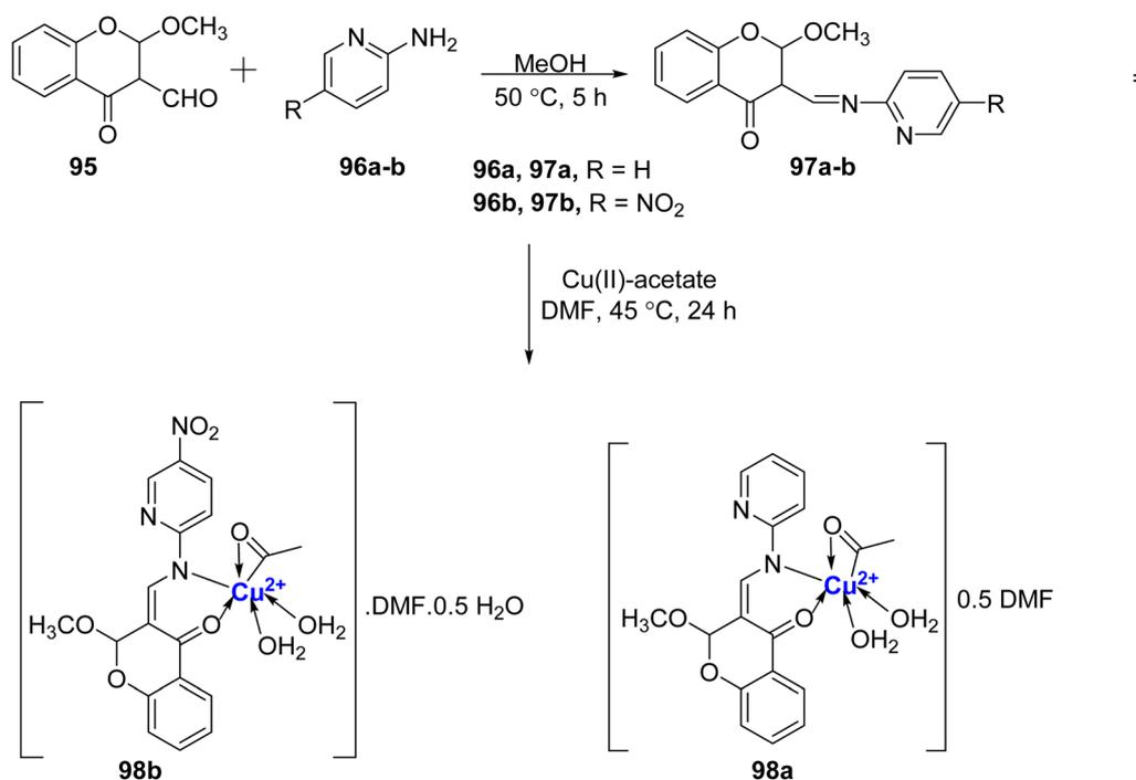
Scheme 28 Synthesis of 2-methoxy-4-chromanone based ligands **97a–b** and its copper(II)-complex **98a–b**.
