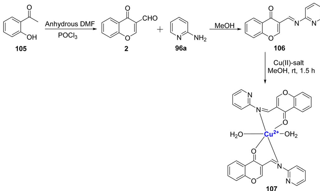
Scheme 31 Synthesis of ligand **106** and its copper(II)-complex **107**.
