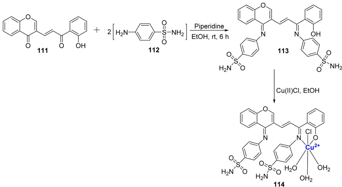
Scheme 33 Synthesis of ligand **113** and its copper(II)-complex **114**.
