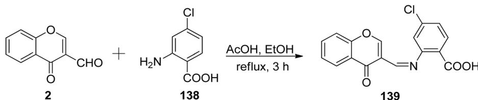
Scheme 42 Synthesis of Schiff base ligand **139**.
