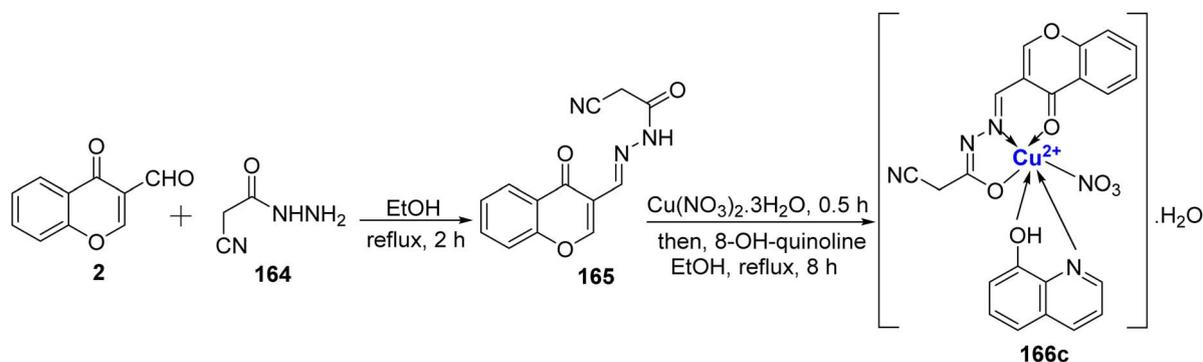
Scheme 50 Synthesis of ligand **165** and Cu(II)-ion complex **166c**.
