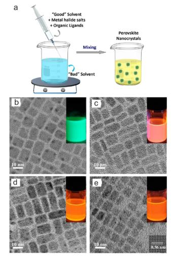
(a) Schematic illustration of supersaturated crystallization method. TEM images of (b) CsPbBr<sub>3</sub> NCs and CsPb(Cl/Br)<sub>3</sub>:Mn<sup>2+</sup> NCs with Mn/Pb molar feed ratios of (c) 2.0, (d) 5.0, and (e) 7.5, respectively. Insets show their PL photographs dispersed in cyclohexane under ultraviolet lamp irradiation. Reproduced with permission from ref. 52. Copyright 2017, American Chemical Society.
