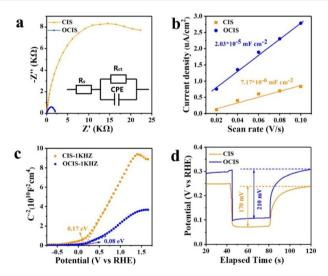
Fig. 5 (a) The EIS Nyquist plots for CIS and OCIS under illumination. (b) Current densities of Cdls of CIS and OCIS. (c) M-S plots for CIS and OCIS in dark. (d) OCP measurements under dark and light conditions for CIS and OCIS
