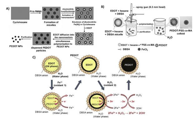
Fig. 3 Different polymerisation synthesis approaches of PEDOT NPs. (A) PI-b-PMMA stabilised NPs in non-aqueous emulsion with cyclohexane and acetonitrile. Reproduced with permission from ref. 61 Copyright 2006 Wiley. (B) Spray emulsion polymerisation of PSS-co-MA stabilised PEDOT NPs. Reproduced with permission from ref. 64 Copyright 2010 Wiley. (C) Fe<sup>3+</sup>/H<sub>2</sub>O<sub>2</sub> bi-oxidant system. Reproduced with permission from ref. 68 Copy right 2011 Elsevier.
