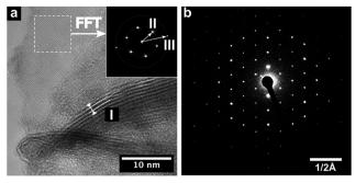
Fig. 5 (a) HRTEM image of pristine WSe<sub>2</sub> flower like structures with interplanar distance of 0.67 nm (a) corresponding to the (002) plane. Fast Fourier transformation (FFT) of selected area yields highly ordered hexagonal pattern (inset) corresponding to the (100) (II) and (110) plane (III), respectively. (b) Hexagonal SAED pattern confirms the high crystallinity of WSe<sub>2</sub> flakes.
