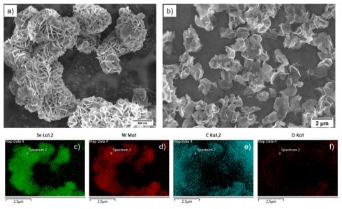
Fig. 4 (a) SEM image of WSe<sub>2</sub> with flower-like arrangement of 2D flakes, (b) SEM image of dispersed WSe<sub>2</sub> flakes, (c)-(f) elemental mapping showing homogeneous distribution of tungsten and selenium located on as-prepared WSe2 structures.
