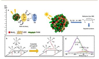
(a) Schematic illustration of the photocatalytic reduction of MB. Reprinted with permission from ref. 139 Copyright 2019, Elsevier. (b) Illustration of the mechanism of TiO<sub>2</sub> on the surface of GO sheet. (c) XPS spectra of TiO<sub>2</sub>-graphene. Reprinted with permission from ref. 140 Copyright 2020, Elsevier.
