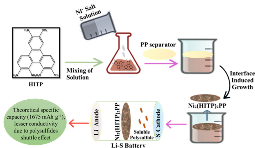
Fig. 6 The application of MOFs in lithium sulfur batteries. 116
