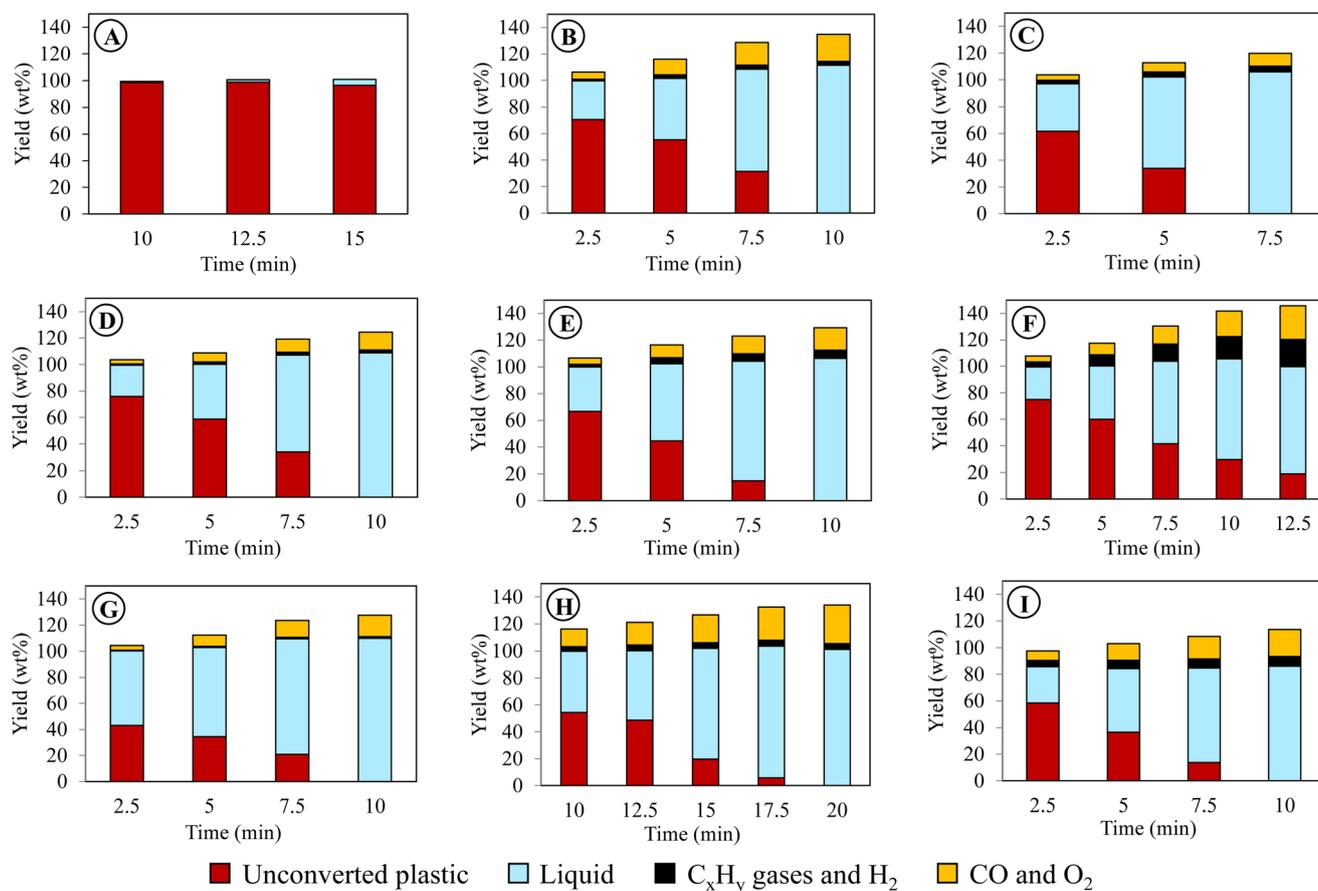
**Fig. 1** Time-dependent product distribution calculated per initial PE mass for different plasma conditions. Refer to Table 1 for the alphabetical nomenclatures in circles and their corresponding reaction conditions.
